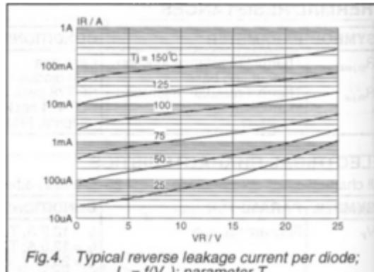
Fig.4. Typical reverse leakage current per diode;
