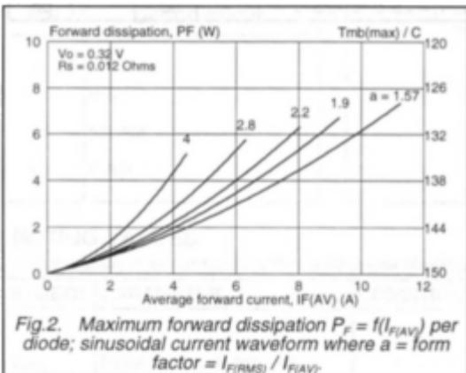
Fig.2. Maximum forward dissipation  $P_F = f(I_{F(AV)})$  per diode; sinusoidal current waveform where  $a$  = form factor =  $I_{F(RMS)} / I_{F(AV)}$ .
