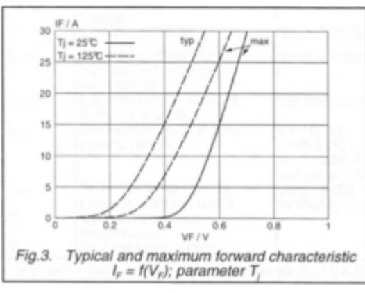
Fig.3. Typical and maximum forward characteristic
