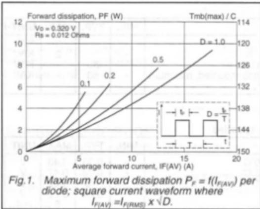
Fig.1. Maximum forward dissipation  $P_F = f(I_{F(AV)})$  per diode; square current waveform where
