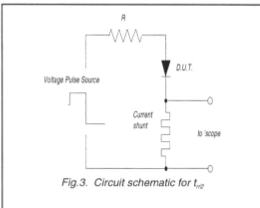
Fig.3. Circuit schematic for  $t_{r2}$
