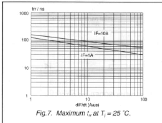
Fig.7. Maximum  $t_{rr}$  at  $T_j = 25^\circ\text{C}$ .
