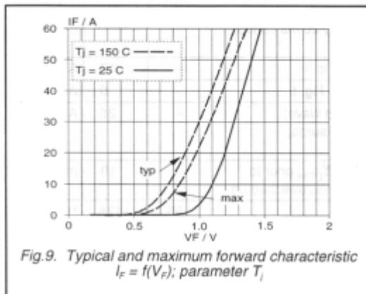
Fig.9. Typical and maximum forward characteristic
