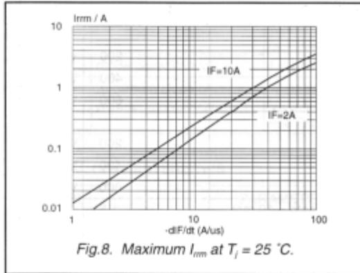
Fig.8. Maximum  $I_{rm}$  at  $T_j = 25^\circ\text{C}$ .
