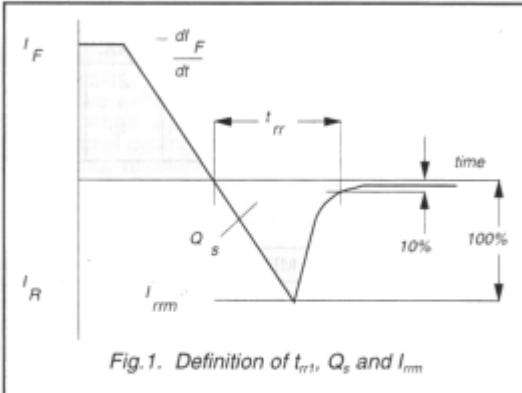
Fig.1. Definition of  $t_{rr}$ ,  $Q_s$  and  $I_{rm}$
