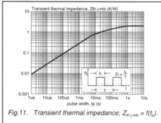
Fig.11. Transient thermal impedance;  $Z_{th,j-mb} = f(t_p)$ .
