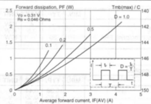
Fig.1. Maximum forward dissipation  $P_F = f(I_{F(AV)})$  per diode; square current waveform where  $I_{F(AV)} = I_{F(RMS)} \times D$ .
