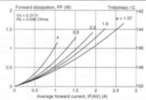
Fig.2. Maximum forward dissipation  $P_F = f(I_{F(AV)})$  per diode; sinusoidal current waveform where  $a$  = form factor  $= I_{F(RMS)} / I_{F(AV)}$ .
